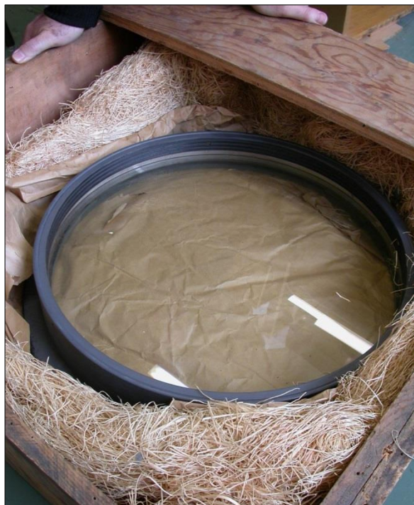
Figure 4: Brashear's 46-cm objective before installation in the restored New Zealand telescope. (courtesy: Adrian Ashford Collection).
