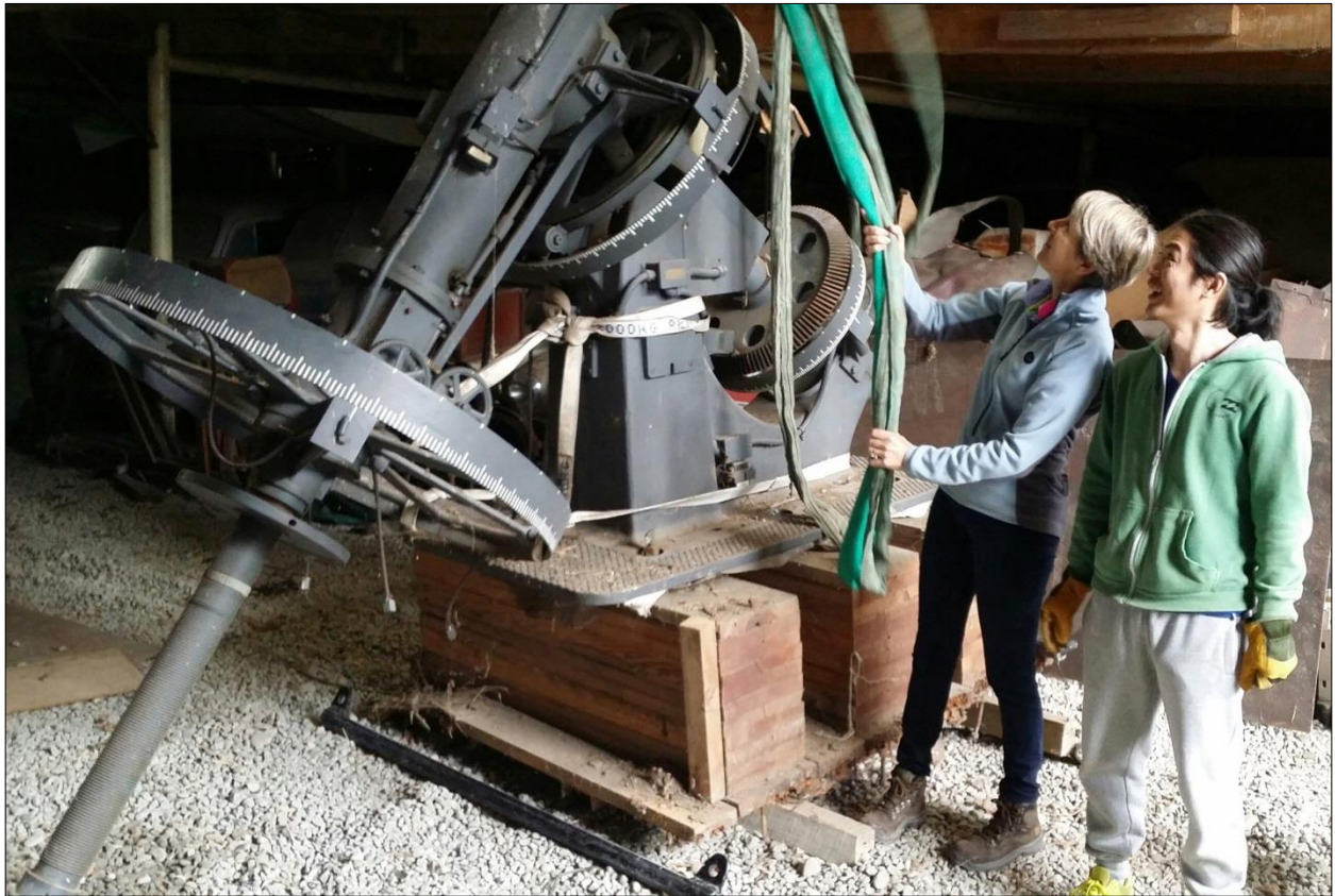
Figure 13: The refurbished Warner and Swasey equatorial mounting in New Zealand (courtesy: Adrian Ashford collection).
